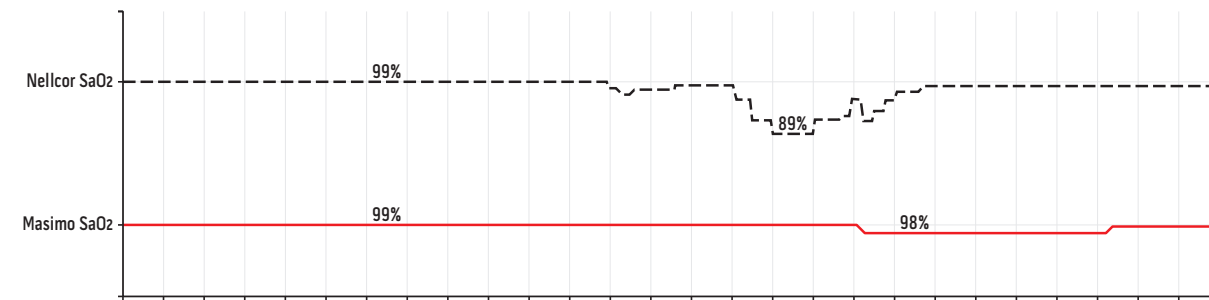
This figure shows a typical type M event, one in which motion caused a false desaturation event on the Nellcor oximeter.
